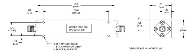
Micro-Tronics Model BPC50301 was specifically designed to pass 3700 to 4200 MHz while maintaining low insertion loss and sharp rejection. The basic bandpass filter design can also be adapted to custom applications.
