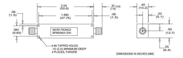
Micro-Tronics Model BPM50603 was specifically designed to pass 225 to 400 MHz while maintaining low insertion loss and sharp rejection. The basic bandpass filter design can also be adapted to custom applications.
