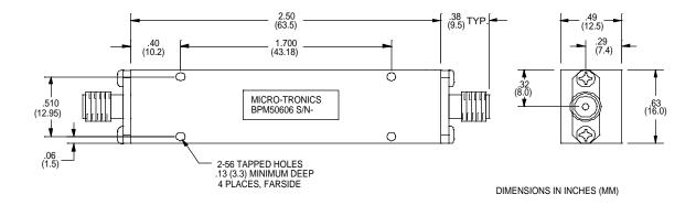
Micro-Tronics Model BPM50606 was specifically designed to pass 1000 to 2000 MHz while maintaining low insertion loss and sharp rejection. The basic bandpass filter design can also be adapted to custom applications.
