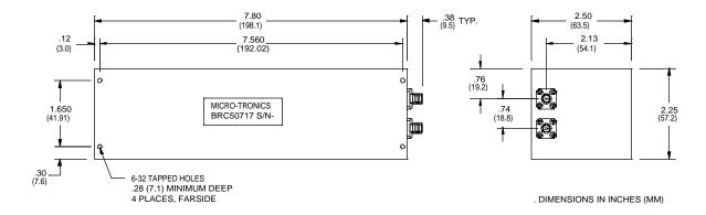
Micro-Tronics Model BRC50717 was specifically designed to reject 825 to 850 MHz while maintaining low insertion loss and broad upper passband. The basic notch filter design can also be adapted to custom applications.
