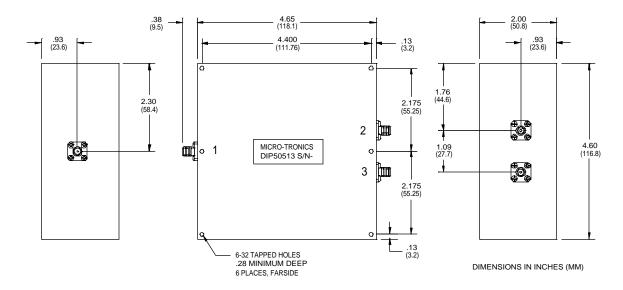
Micro-Tronics Model DIP50513 was specifically designed to pass 880-915 MHz and 925-960 MHz (EGSM band) while maintaining low insertion loss and sharp rejection. The basic Diplexer design can also be adapted to custom applications.
