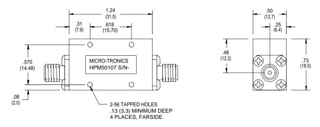
Micro-Tronics Model HPM50107 was specifically designed to reject DC to 7200 MHz while maintaining low insertion loss and a broad upper passband. The basic highpass filter design can also be adapted to custom applications.
